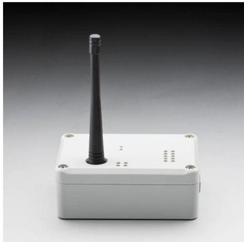
The GatewayNode radio radio radio opens a new segment on an existing segment (via the radio interface). A normal segment can be extended a maximum of once with a repeater, but two independent GN.R can be connected to a normal segment (Y shape).
