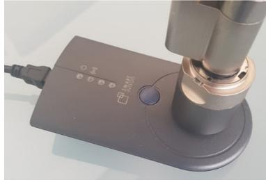
During programming via WaveNet, the SI.SmartCD only needs to be connected to a free USB port until the first locking device has been programmed. The configuration is then fully saved in the SmartIntego tool and the SI.SmartCD can be removed. However, as soon as the card configuration has been changed, the SI.SmartCD must be connected once. It can then be removed again after programming the first locking device.
